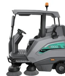
TS1900H is a powerful and large semi-enclosed ride-on floor sweeper machine, designed for large-area indoor and outdoor industrial sweeping tasks. With manual trash can, it's suitable for daily sweeping in areas such as airport stations, parking stations, large-scale logistics warehouses, production workshops, etc.
